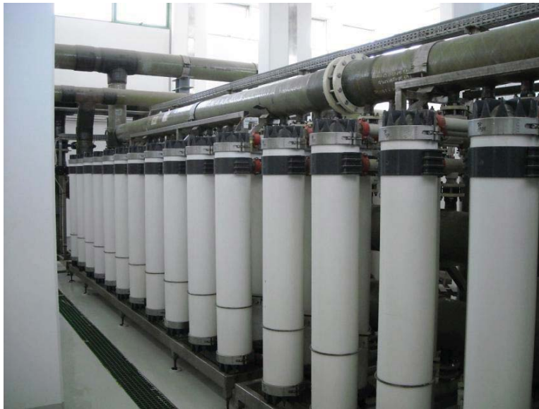
Photo: The ultrafiltration system in Abu Dhabi supplied by inge watertechnologies AG will treat 80,000 m 3 of water a day.
